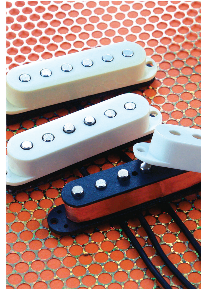
CST-N #11301W Neck Alnico 5 ROD 2P Shield 5.6K CST-C #11302W Center Alnico 5 ROD 2P Shield RWRP / 5.8K CST-B #11303W Bridge Alnico 5 ROD 2P Shield 6.4K
